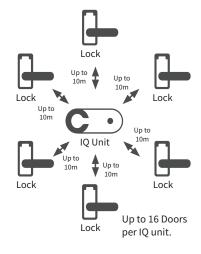
Adding a repeater allows you to extend the distance between the IQ unit and your locks by up to 10 meters. You may add up to 6 repeaters in between an IQ unit and a lock which means that the maximum distance between a door and the IQ unit is up to 40 meters.
